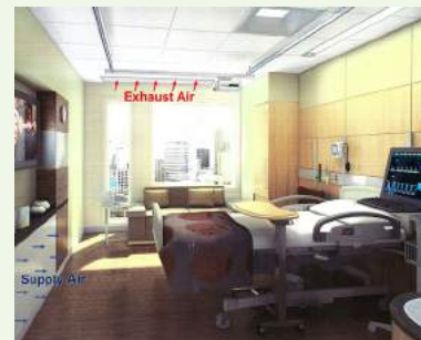
▼ FIGURE 3: Displacement Ventilation System
